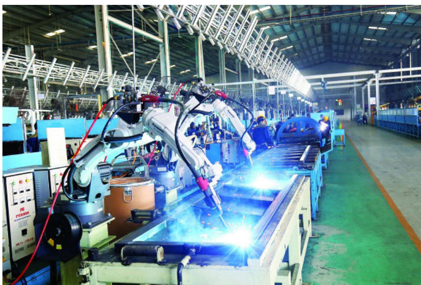
Figure 2: Robot welding technology at Mechanics Company (THACO)
