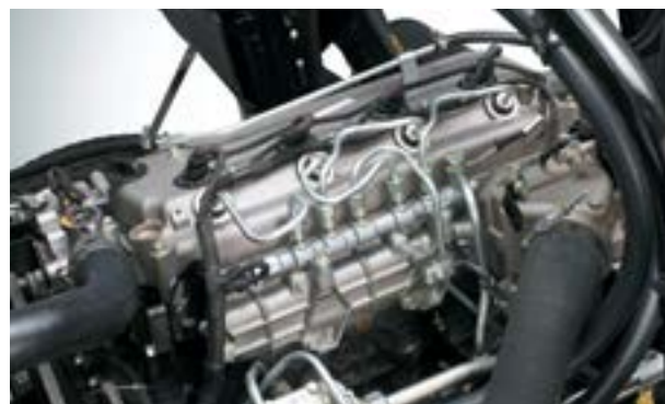
The truck is equipped with Mitsubishi engine with CRD-i direct injection, offering power, fuel-efficiency and environmentally friendliness.
