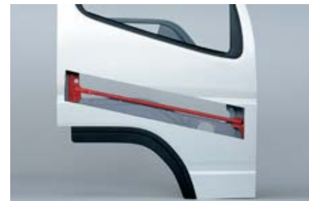
Reinforcing bars on the doors increase safety for drivers and passengers in case of collisions
